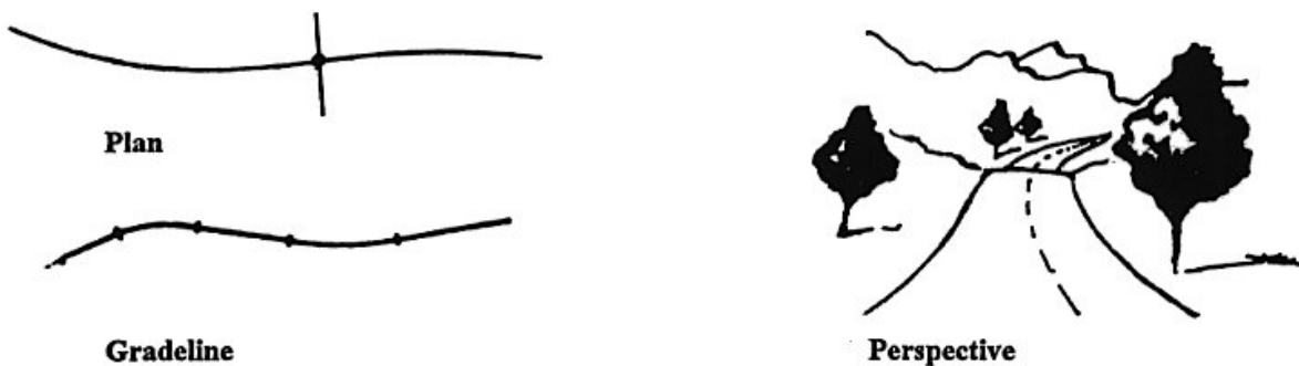
Figure 6.4: Intersection hidden behind a crest (poor design practice)
