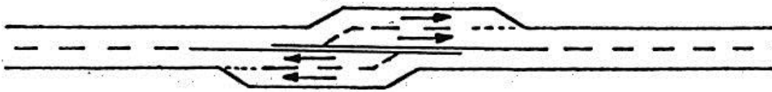
OVERLAPPING OVERTAKING LANES - After location.
