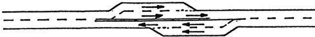
OVERLAPPING OVERTAKING LANES - Before location
