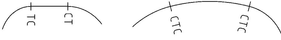
Figure 7.2: Types of broken back curves
