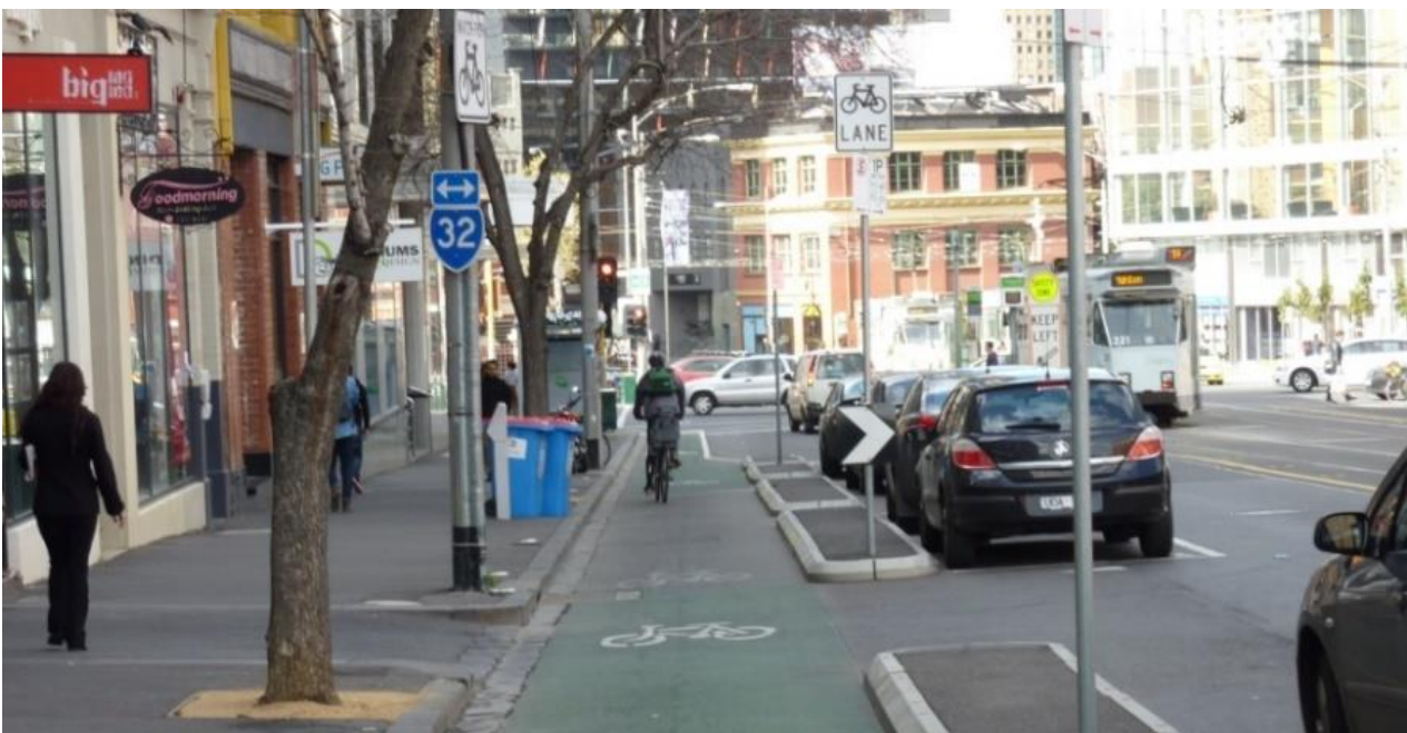
Figure 4.40: Separated bicycle lane with physical separation of parking (Swanston Street, Melbourne)
