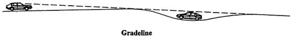
Figure 6.6: Shallow dip (poor design practice)
