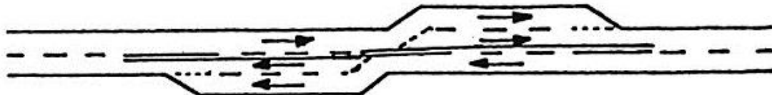
ADJOINING OVERTAKING LANES - After location
