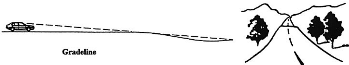
Figure 6.6: Shallow dip (poor design practice)
