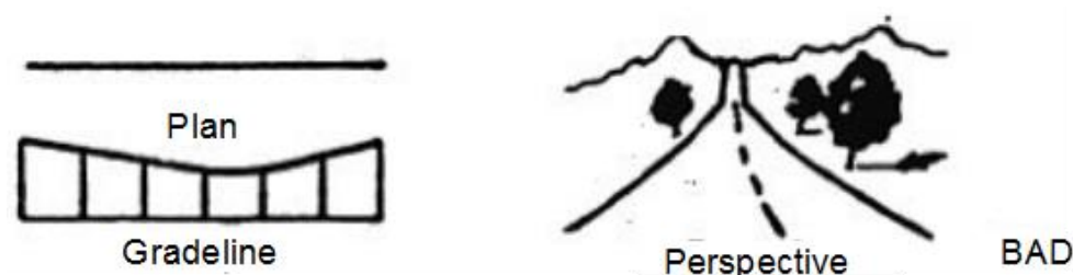
Figure 6.15: Short sag curve appears kinked
