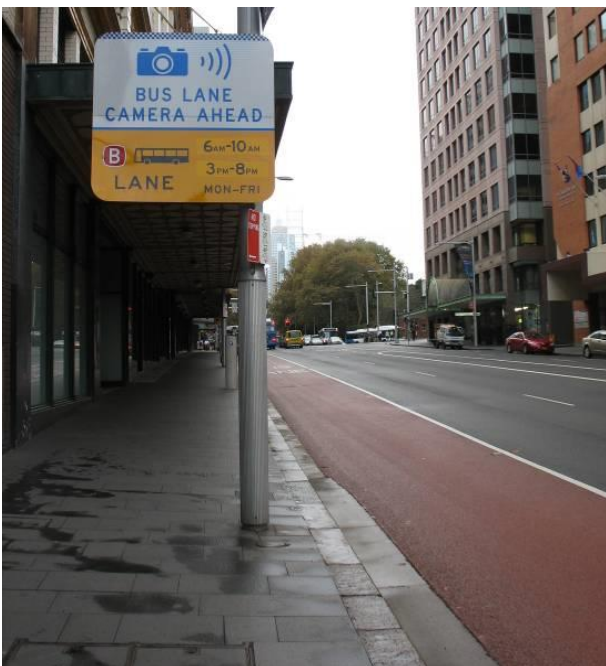
Figure 4.43: Example of a camera systems to record illegal use of bus lanes
